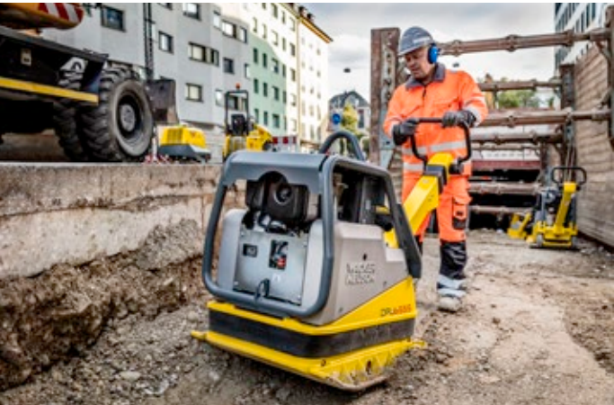
Safe in every case: If the guide handle is released, the unit only vibrates on the spot.
