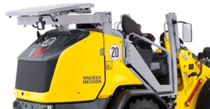
Folded down quickly: the EPS (Easy Protection System) operator's canopy.
