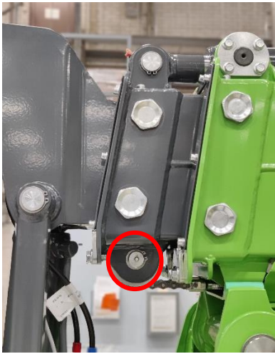
Figure 18. Telescope chain pulley wheel greasing point at the work platform end
