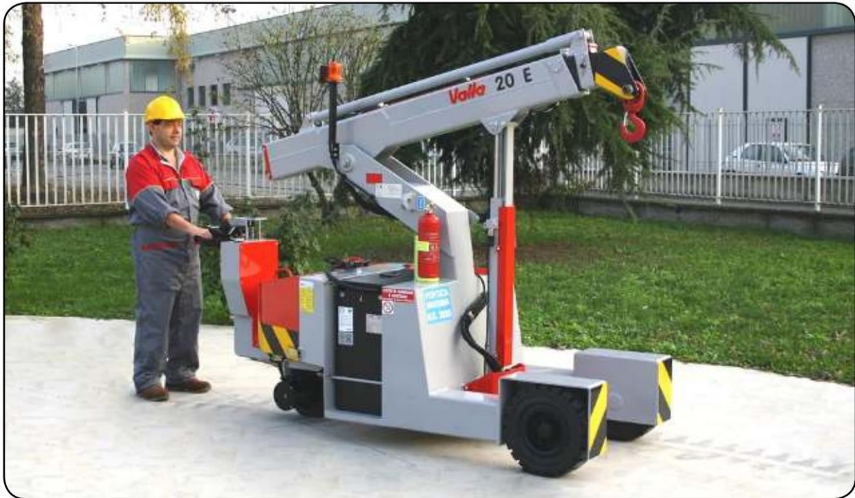
**PROPULSION:** 2 kW - 24 V AC fanned reversible electric motor fitted with electronic speed control. Disk brake on drive wheel electrically operated. Equipped with dead man cut out. Reduction between motor and wheel by gears in oil bath. Max speed 3,5 Km/h.
