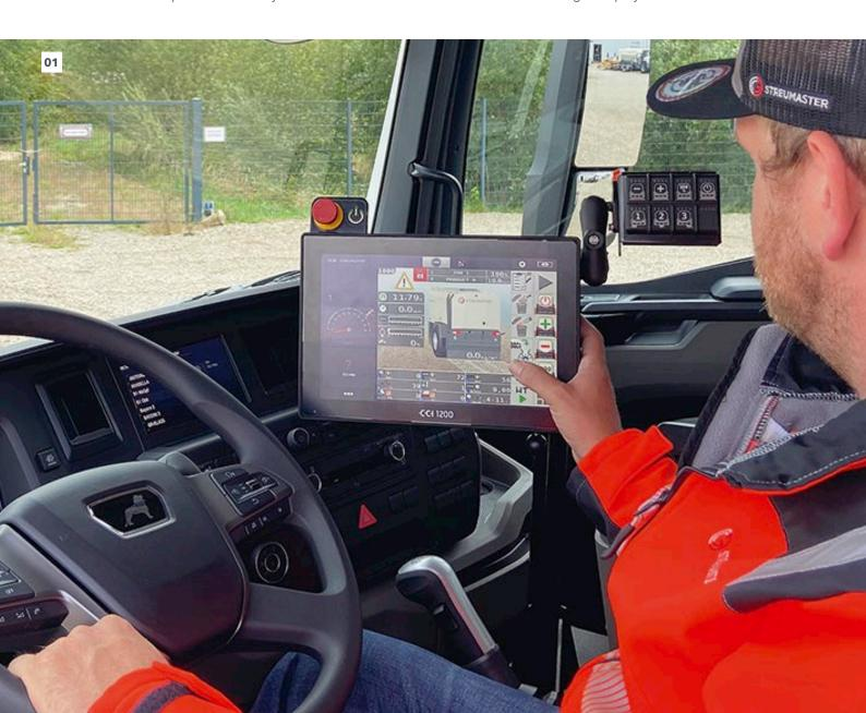
is available in conjunction with the WeighTronic option. This display makes it possible to read and check the weight of the binding agent in the container from the outside at any time during the filling process.
