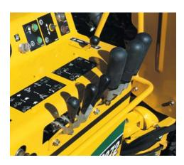
Operator presence system. The SC372 is equipped with three operator-sensing control levers that monitor the operator's touch and maintain cutter wheel engagement. When the operator's hands leave the control levers, an automatic disengage and braking sequence will stop the cutter wheel in less than nine seconds. With this safety system, the cutter wheel will automatically stop when the operator releases the hydraulic cutter wheel controls.
