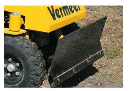
An optional chip blade helps eliminate the need for manual chip raking during jobsite cleanup. The blade is controlled hydraulically from the operator's station.
