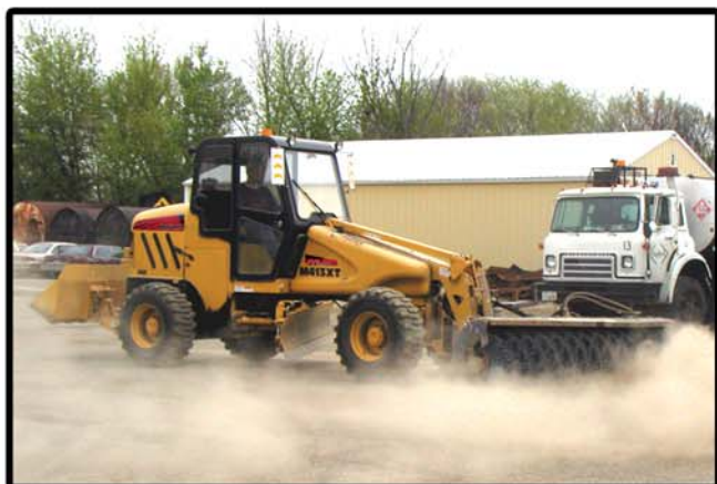
M413XT with 84 inch Broom Attachment adds versatility and productivity to this work horse.
