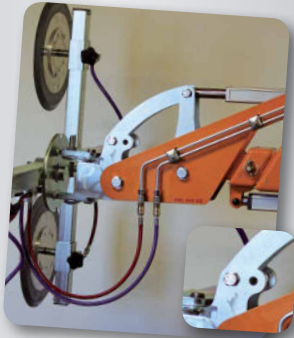
The lifting head has two settings, adjusted by means of two holes for the locking bolt. The lifting head can therefore be adjusted to tilt more towards the ceiling or floor.
