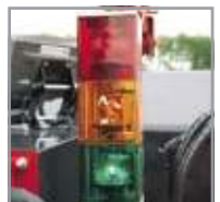
Overload warning lamps + auto stop + alarm
