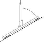
upright or the flat position, the load force on the control handle changes direction during the tilt. If load size permits, maintain control with the handle throughout the tilt. For loads with overhang, it may be necessary to release the control handle as the load approaches the flat position. If so, keep the load under control using hand cups or other appropriate means.
