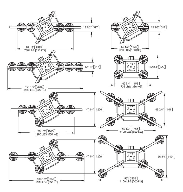
Configurations are created by installing or removing the pad frame's <u>extension arms</u>, by repositioning or removing the <u>movable pad mounts</u>, and by connecting or disconnecting the vacuum hoses to certain <u>vacuum pads</u>. Always assemble the pad frame in a symmetrical arrangement, to keep the lifter balanced (see illustration).
