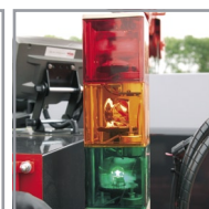
Overload warning lamps + auto stop + alarm
