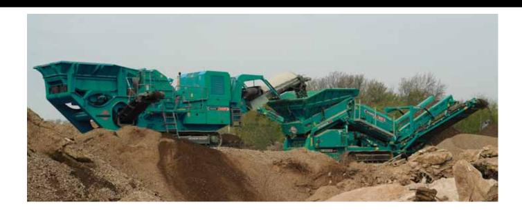
The Powerscreen® Warrior 1400 is a flexible screening machine, aimed at small to medium sized operators who require a high performing, heavy duty, versatile machine that remains easy to transport. Its highly aggressive screen can accept bofor bars, finger screens, woven mesh and punch plates.
