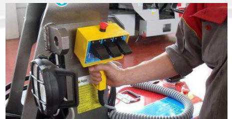
Wired remote control for the aerial part
