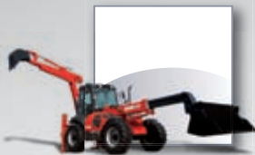
MANIHOE Backhoe/Loader with telescopic boom
